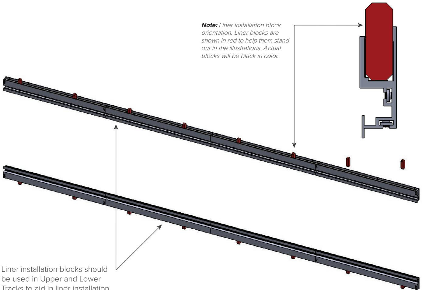
Liner installation blocks should be used in Upper and Lower Tracks to aid in liner installation.
