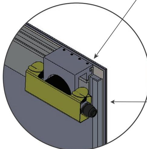
The body of the Carriage **MUST** be installed flush with the end of the mounting track as shown. Make sure the left and right side Carriages are installed on the correct side. The Bumper should point to the outside of the sliding panel when installed correctly.
