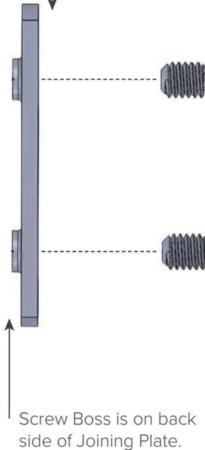
1. Once the first section is installed, install the remaining Standard Wall Sections for the Upper Track, so that when completed — there are the same number of sections on either side of the vertical system center laser line.
